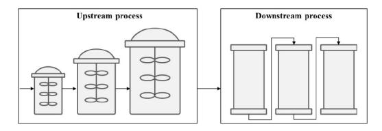
**Figure 2:** Schematic view of a biopharmaceutical production process with a singular serial seed-train and three sequential chromatography columns
