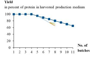
**Figure 4:** Deterministic performance decay pattern of a candidate chromatography resin over 11 purified batches, with selected stochastic decay scenarios starting after the fifth batch, adapted from Liu et al. (2014)
